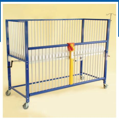
New, easy to operate handle! Turn handle and lift to unlock the side rail, then lower. To raise, just lift the side rail and it locks securely at two mid-stops and fully closed position.
